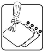
5. Replace the battery cover and tighten the screw to secure.
